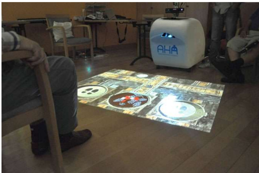
Fig. 1 PEPE consists of a wheeled mobile platform with a depth sensing camera and floor projection capabilities. It delivers a customizable exercise program through gamified activities and physiological adaptation that can be used through full-body interaction
