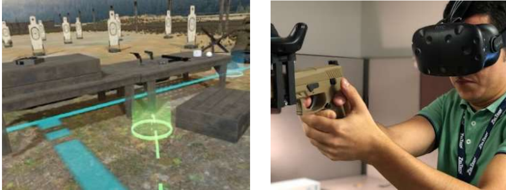
Figure 44. BioPhyS simulator developed for the J&F Alliance company under the supervision of Dr. Alan Pope from NASA Langley. Left: screenshot of the VR simulation. Right: picture of one test carried out to integrate airgun weapons.
