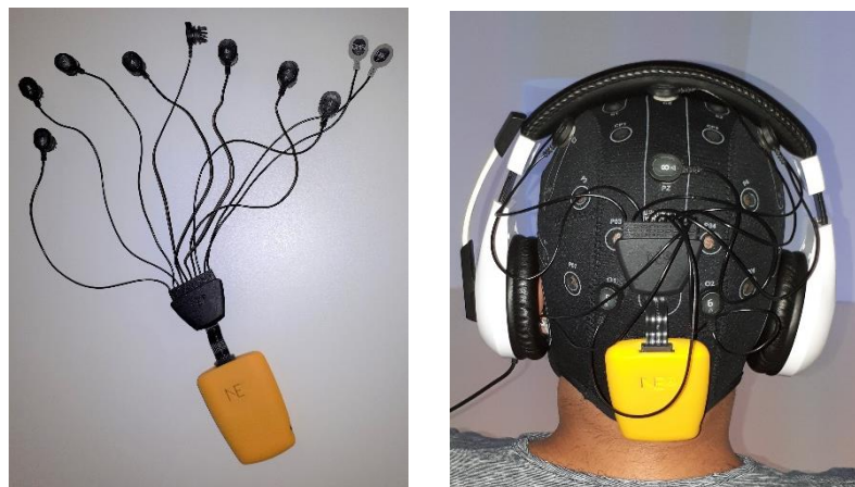
Figure 4.4 On the left, the Enobio8 system. It has 8 EEG channels and 2 reference channels. On the right, a participant wearing the neoprene cup with the Enobio device attached. The headphones were used for sound isolation during the NF training session.
